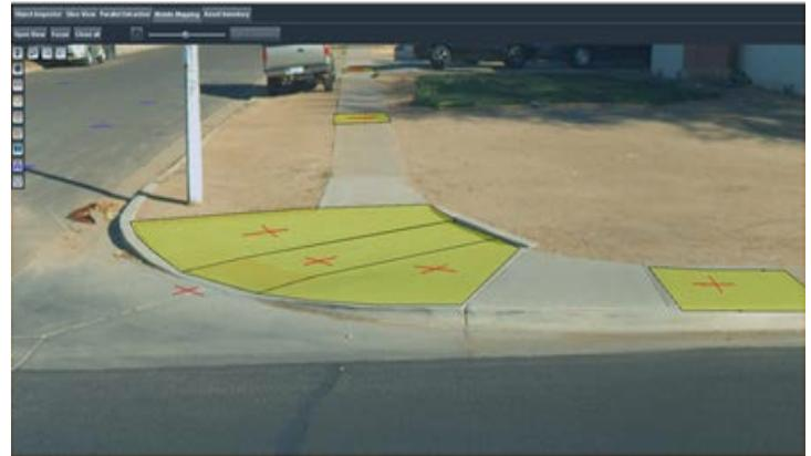
Ramp and Sidewalk features with running slope and cross slope lines.
